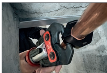
180° swivel increases flexibility in operations in tight spaces
