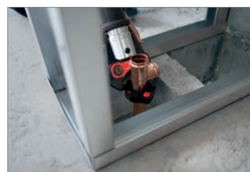
No press ring swap required between standard and compact actuator jaw
